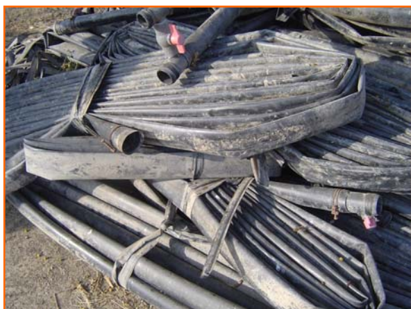
Figure 2. Thin walled drip irrigation sub-mains and driplines in Hyderabad, Pakistan (imported materials from China).
