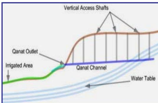
**Figure 12. Qanat/Karez system schematic**
